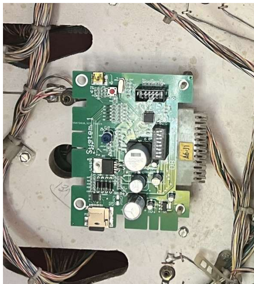
Figure 1 - Ni-Wumpf replacement sound board installation – System 1 vs System 80
